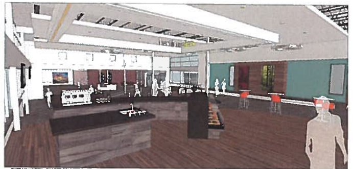
CAFE MILLWORK - QUARTZ COUNTERS WITH PLASTIC LAMINATE CABINETRY CAFE EQUIPMENT BY OWNER
